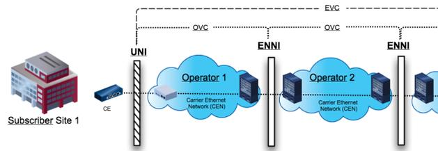
From the diagram it can be seen that there are two types of operator interconnections in a service that crosses a multi-CEN network. One type of operator can contain a UNI and an ENNI. The other type of operator has two ENNIs—this is a transit operator. (Note that each operator could have more than one UNI and/or more than one ENNI supporting a multipoint service).
