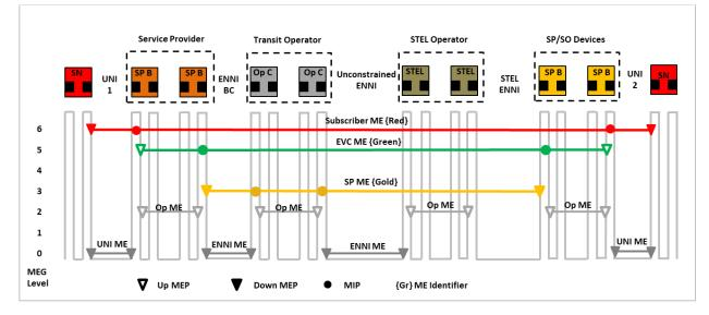
Figure 8 – Example of SOAM with Two SP/SO Devices
