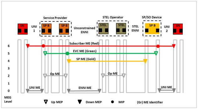
Figure 7 – Example of SOAM with a SP/SO Device
